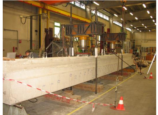
Fig. 1. Experimental set-up for creep test on precast beams (Mazzotti).
