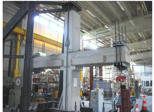
Fig. 2. Cyclic loading test on beam-column node in full-scale (Mazzotti).
