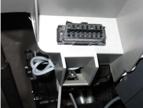
Fig. 4. Common OBD-II port.
