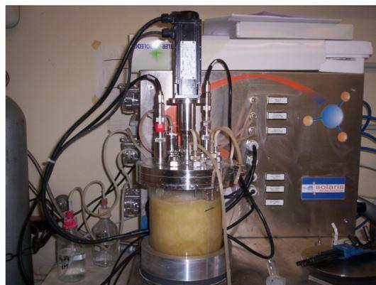
Fig. 2. Fermenter for bioconversion to biovanillin.
