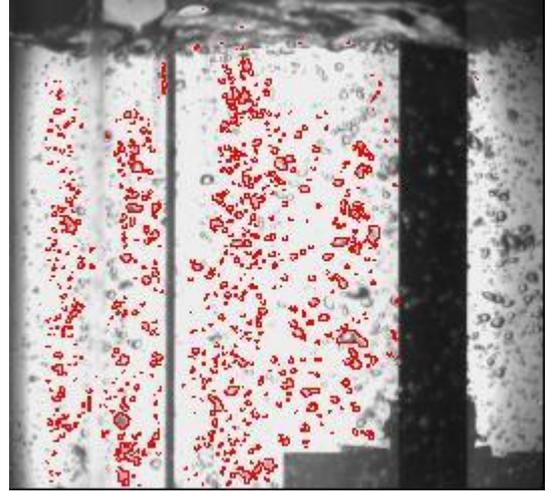
Fig.1 Multiphase stirred tank: bubble size analysis.
