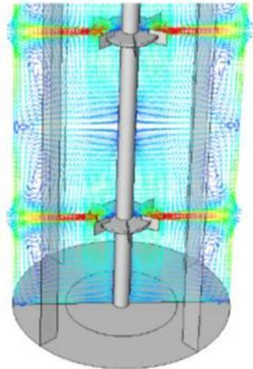
Fig.2 CFD simulation of a stirred tank: the flow field.
