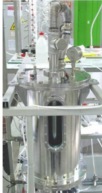
Fig. 1. Bioreactor for the biological production of hydrogen.
