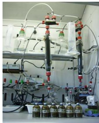
Fig. 2. Bioreactors for the biomethanization of organic wastes.
