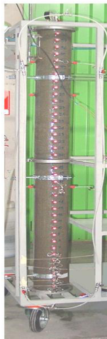
Fig. 1 Attached-cell bioreactor for the treatment of groundwater.
