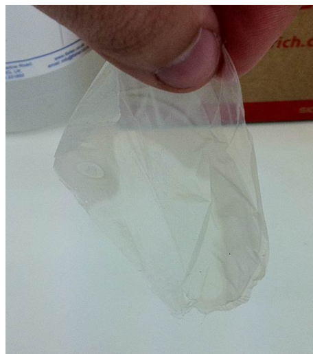
Fig. 1. PHA film obtained by chemical extraction of the polymer from C. necator culture
