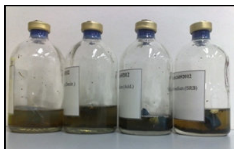
Fig. 2. Anaerobic microcosms for the enrichment of microbial communities from waste plastics able to degrade synthetic polymers.
