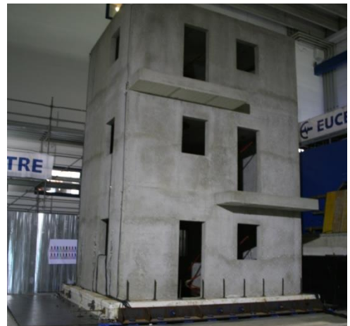
Fig. 3. Tests on a full-scale 3-storey building realized with RC sandwich panels, at the EUCENTRE.
