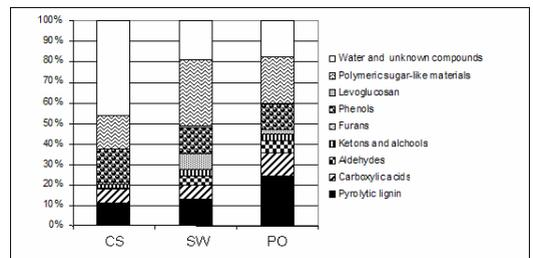
Fig.2 Example of pyrolysis products from different biomass types.
