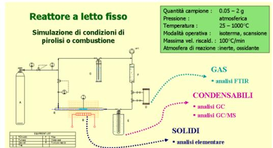
Fig.1 Fixed bed reactor for experimental characterization of feedstock
