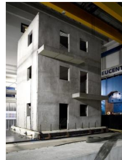
Fig.3 Shaking-table tests upon a full-scale 3-storey building (Silvestri).
