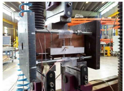
Fig. 3. Shear test on masonry triplet. Precompression apparatus (Gentilini).
