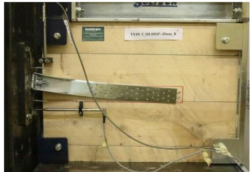
Fig. 2. View of a specimens tested with combined tension-shear forces (Pozza).
