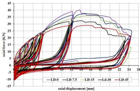
Fig. 3. Cyclic behaviour of steel to timber connection with different level of tension-shear interaction (Pozza).
