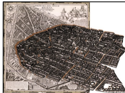
Fig. 2. Digital processing and 3D modelling from an 18th century scenographic map of Bologna (Bitelli & Gatta, 2011).
