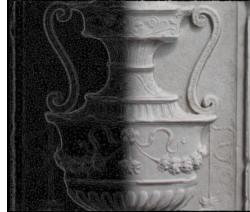
Fig. 1. Structured-light projection scanning for 3D modelling (from the “Colonna dei Francesi”, Ravenna). Left: wireframe view; right: photo-textured view, (picture by Bitelli).
