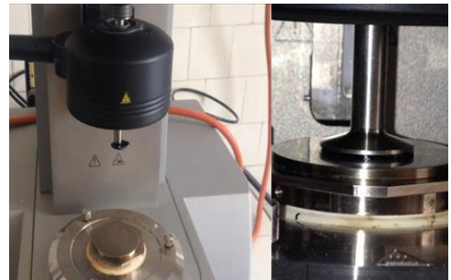
Fig. 1. Dynamic Shear Rheometer testing on rubberized bituminous mastics.
