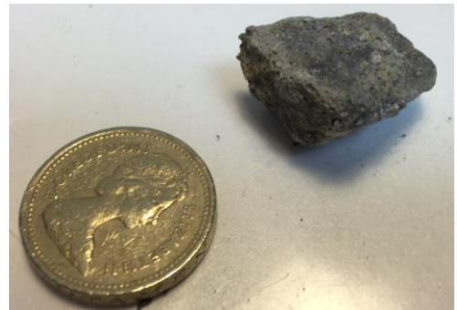
Fig. 2. Artificial engineered aggregate made of alkali-activated waste materials.
