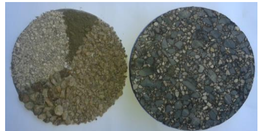
Fig. 3. Recycled waste bleaching clays (dark brown) in an asphalt concrete aggregates gradation.
