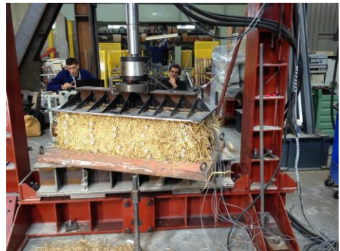
Fig. 3. Compressive test on straw bale (Molari).
