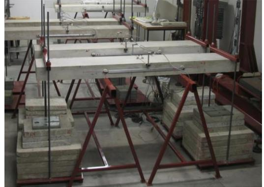
Fig. 1. Long-term tests on cracked FRC beams (Buratti).
