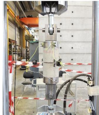
Fig. 2. Uniaxial tension test on notched FRC specimens (Buratti).
