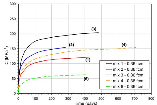
Fig. 3. Development with time of creep for different SCCs (Mazzotti).
