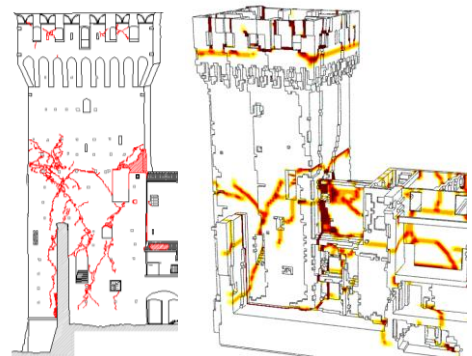
Fig. 3. Nonlinear Response History Analyses (RHA) using natural accelerograms of the San Felice sul Panaro (Italy) fortress, hit by the Emilia earthquake in 2012 (Castellazzi).
