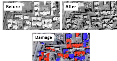
Fig. 4. Bam earthquake (2003): buildings damage mapping through object-based classification of high resolution satellite imagery, (Gusella et al., 2005).
