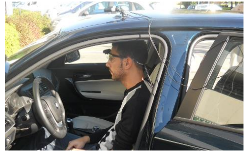
Fig. 1. Mobile Eye-XG glasses for examination of human eye movement and pupil dynamics- installation.
