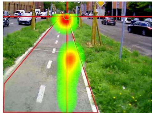
Fig. 1. Exploring the role of gaze behavior and object detection (heat map) in bicycle path understanding and design.
