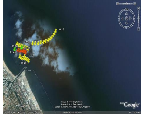
Fig. 1. Sea trajectory monitoring described by oil spill drifters. Measurement campaigns carried out in the coastal area facing Cesenatico between June and September 2009.
