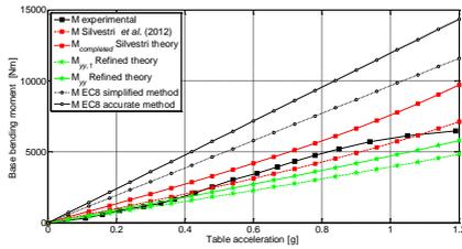
Fig. 4. Comparison between the experimental overturning moment and the predicted values by the theory and by the Eurocode 8 methods (Silvestri).
