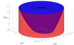
Fig. 2. The red portion is the amount of grain that is completely sustained by the lateral walls of the silo (Silvestri).
