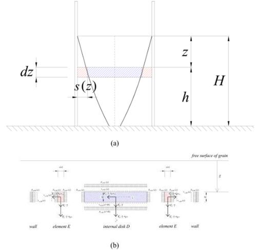
Fig. 1. Vertical longitudinal section of the silo model and forces (Silvestri).
