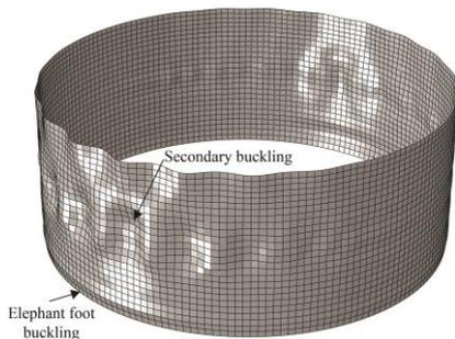
Fig. 5. Numerical simulation of the buckling of a cylindrical tank during a ground-motion (Buratti).
