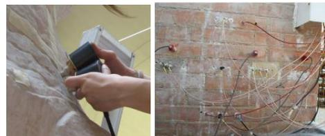
Fig. 3. Ultrasound tests at the David and wireless monitoring of salt content in masonry (Colla).
