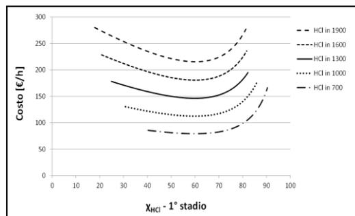
Fig. 2 Economic process optimization of the flue-gas treatment section of a MSWI.
